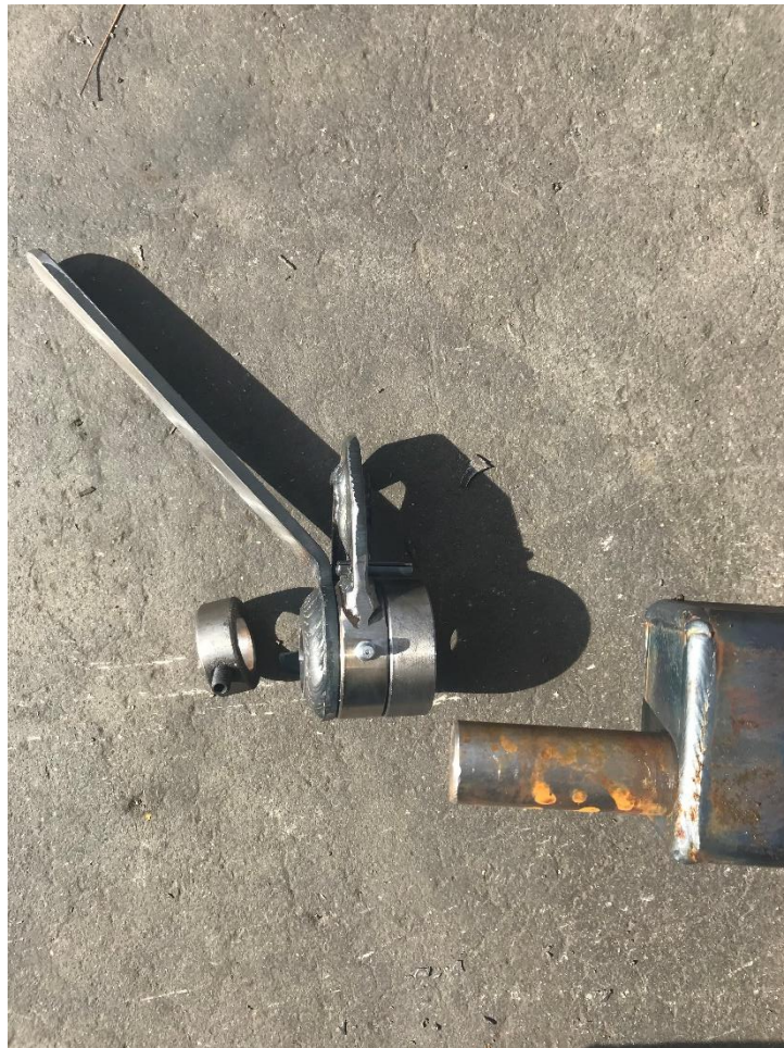
Cam Assembly. The small shaft collar goes on the outside of the assembly when mounted on the post. It is tightened on with the set screw.
