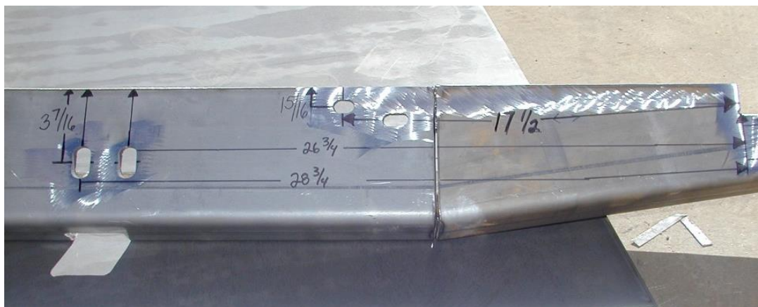
Early Bronco Bumper approx. cutting specs.
